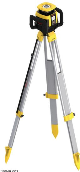
1. Set up the tripod.
