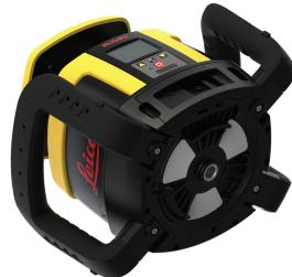
For layout work, use the beam down mode to position the beam over a reference point. Then use the scan mode to move the small scan quickly to a position to the left or right of the Rugby. Alternatively, press beam down to stop the rotating head (0 rps). Refer to [4.3.2 Menu Set 1-Head speed](#).
