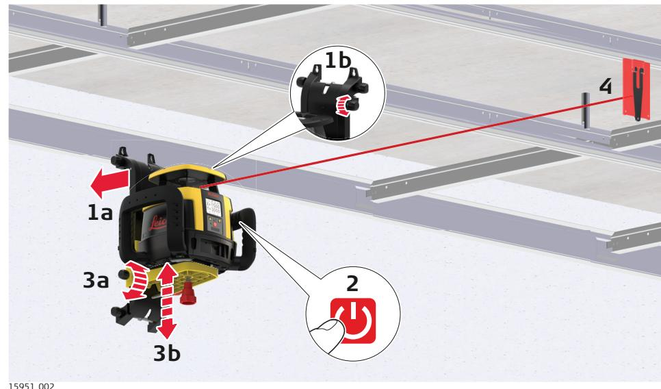
1. After mounting the first strip of ceiling trim at the desired height (centre position of the ceiling target) below, attach the SmartAdapter and Rugby to the trim. Tighten the locking knobs on the top of the SmartAdapter.
