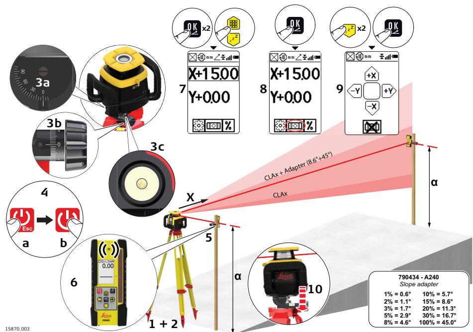
1. Set up the Rugby and the slope adapter on a tripod.
