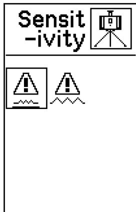
While in use, the Rugby responds to disturbances, for example wind or vibrations, and stops the head rotation, if necessary. You can choose between two levels of sensitivity:
