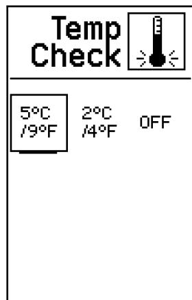
For each change in temperature of  $\pm 5^{\circ}\text{C}$  ( $\pm 9^{\circ}\text{F}$ ) the Rugby returns to the level position to check if the change in temperature has led to a change of the main levelling system. For a more sensitive unit, you can change the setting to  $\pm 2^{\circ}\text{C}$  ( $\pm 4^{\circ}\text{F}$ ) temperature change.
