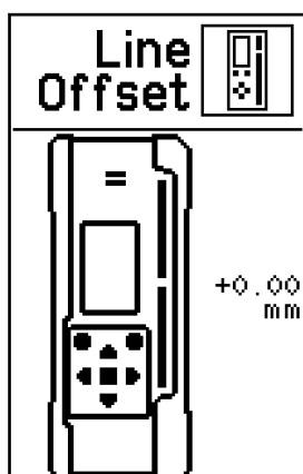
1. Move the Combo+ so the beam is on the desired centre line position.
