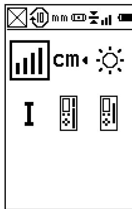
If there is no Rugby paired with the Combo+ a reduced menu screen is shown. This menu is limited to features that do not require an active connection to a Rugby.
