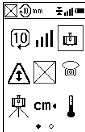
When the Rugby is operated lying on its side the beam down mode is activated automatically.
