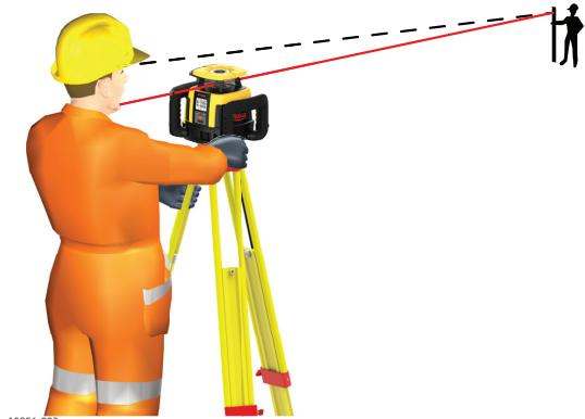
3. Rotate the Rugby slightly until the alignment marks are aligned with your second control point.
