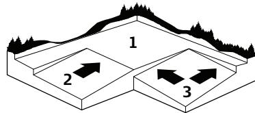
The Rugby, depending on the configuration, is a dual grade laser. The laser produces an accurate plane of laser light for applications which require level (1), single slope (2) or dual slope (3).
